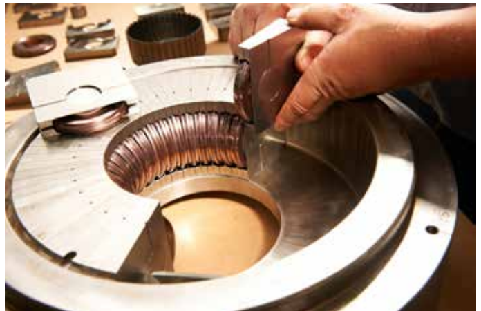
Roller die - at the core of the technology are forming rolls - arranged in pie-shaped cassettes encapsulating a part 360 degrees.
